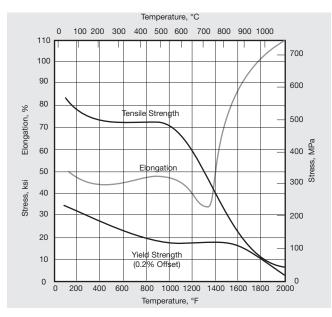
**Figure 1.** High-temperature strength tensile properties of INCOLOY alloys 800H and 800HT.
