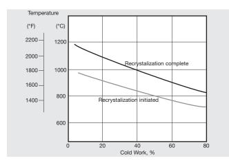
Figure 11. Effect of cold work on recrystallization of alloys 800H and 800HT (UNS N08810 and N08811)
