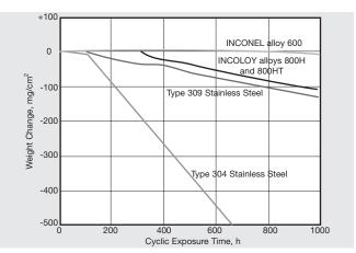
Figure 8. Results of cyclic oxidation tests at 1800°F (980°C). Cycles consisted of 15 min heating and 5 min cooling in air.
