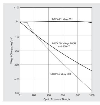
Figure 9. Results of cyclic oxidation tests at 2000°F (1095°C). Cycles consisted of 15 min heating and 5 min cooling in air.
