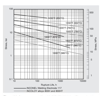
**Figure 14.** Stress-rupture life of INCONEL Welding Electrode 117 as compared with that of INCOLOY alloys 800H and 800HT
