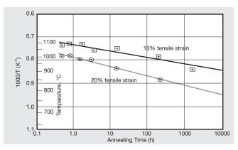
Figure 12. Time at temperature for the onset of recrystallization in INCOLOY alloys 800H and 800HT (UNS N08810 and N08811)
