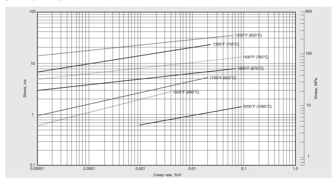
Figure 5. Typical creep strength of INCOLOY alloys 800H and 800HT.
